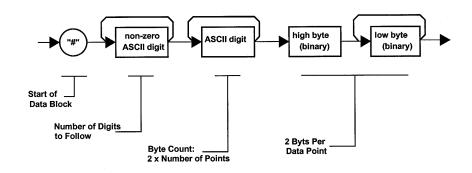
Figure 3. 15, Definite Length Arbitrary Block Data Format
