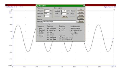
Figure 3.19c Using equation editor to generate five cycles of sine wave
