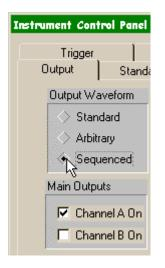
Figure 3. 25 Selecting Sequence output mode
