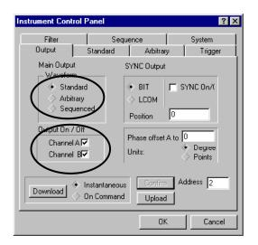
Figure 3.6 Output Control with a WaveCad Panel.
