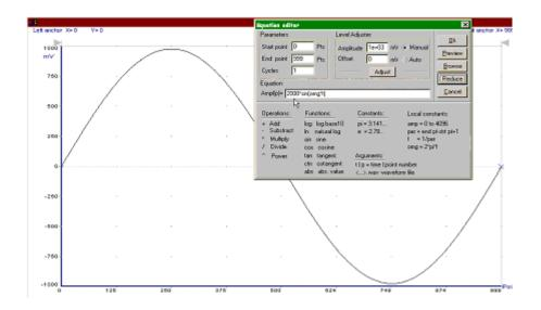
Figure 3.19b Using equation editor to generate one cycle of sine wave with a higher amplitude
