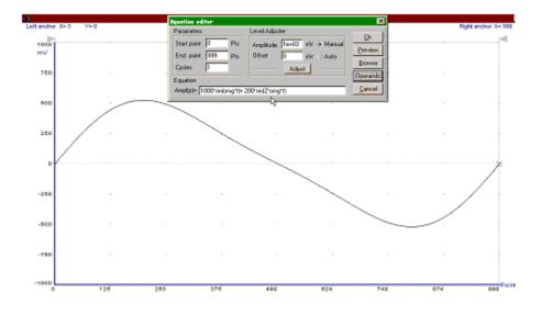
Figure 3.19e Using equation editor to add second harmonic distortion to sine wave
