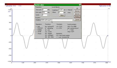
Figure 3.19d Using equation editor to generate five cycles of sine cubed wave
