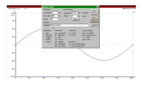
Figure 3.19a Using equation editor to generate one cycle of sine wave
