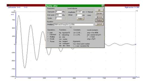
Figure 3.19f Using equation editor to generate exponentially decaying sine Wave
