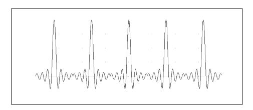
Figure 1.1a , Segment 1 – Sin (x)/x Waveform
