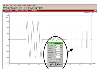
Figure 3.18 Arbitrary waveform made by combining some standard waveforms. The pop-up menu for each wave allows definition of all waveform attributes
